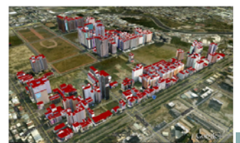
Line-segment digitization, 3D building model reconstruction, automatic façade texture mapping, and export to KMZ.
