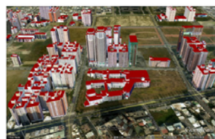
Line-segment digitization, 3D building model reconstruction, automatic façade texture mapping, and export to KMZ.
